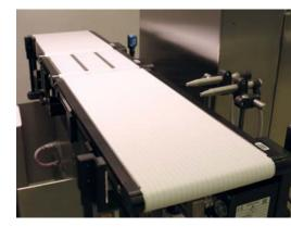
Air blast nozzle (on the right) for secure ejection of under or overweight products
